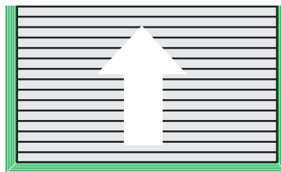
Ramped Edge three-sided. The ramp is NOT connected to the mat but can be secured to the floor.
