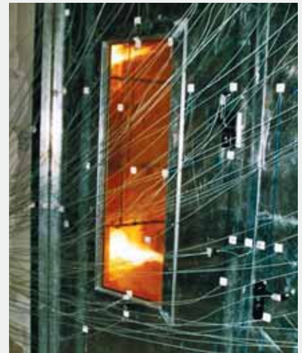
Fire test with temperature measuring devices.
