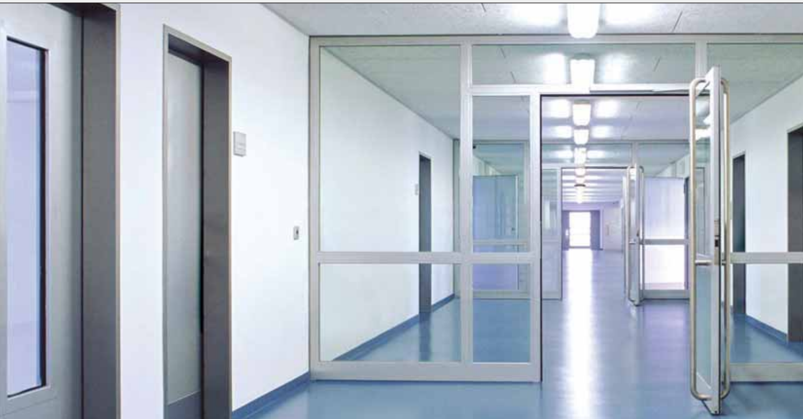
Aluminium smoke-proof door "Schüco ADS 65.NI SP" with side elements and top light.
