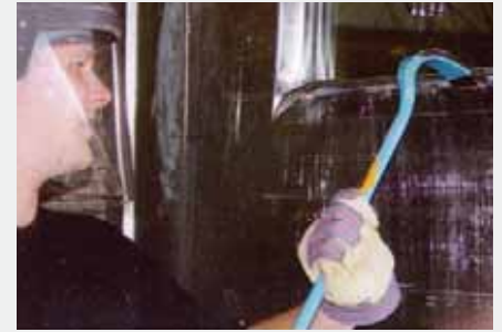
Security test in accordance with ENV 1627.
